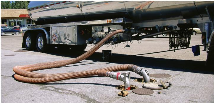
In addition to spills from product delivery, leaks can occur from one or more areas of a storage tank system. Common areas where leaks can occur include underneath the dispenser island, from the spill bucket, from submersible pumps, along the piping that conveys the fuel from the tank to the dispenser, from UST system sumps, and from the tank itself.
